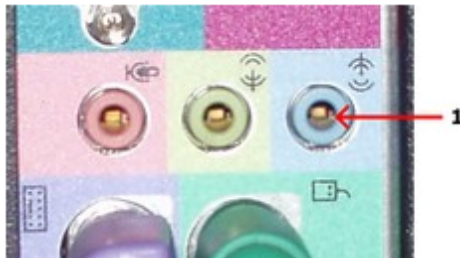
The back pane of a computer with an integrated sound card and a line in mini jack connector (1).
